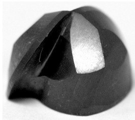
Fig. 8. The spherical part of machined ball-end mill.
